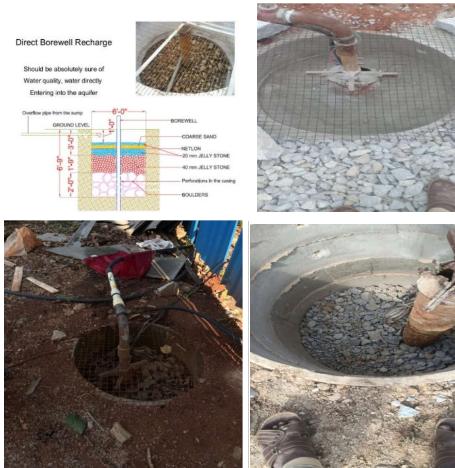
Water Recharge Pits for collection of Rain water
