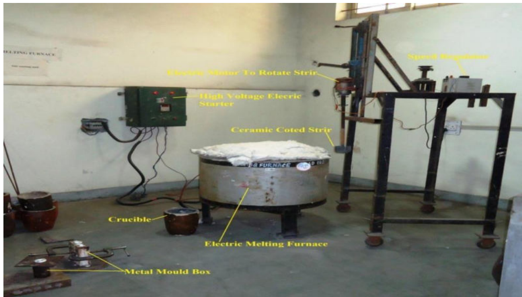
Fig 4.1: Electric al Resistance Furnace for Melting AlSi6
