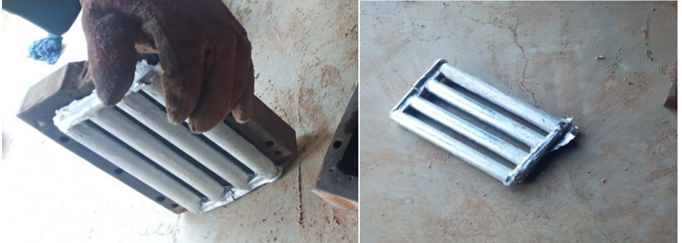
Fig:9 Shows removal of casting from the mold
