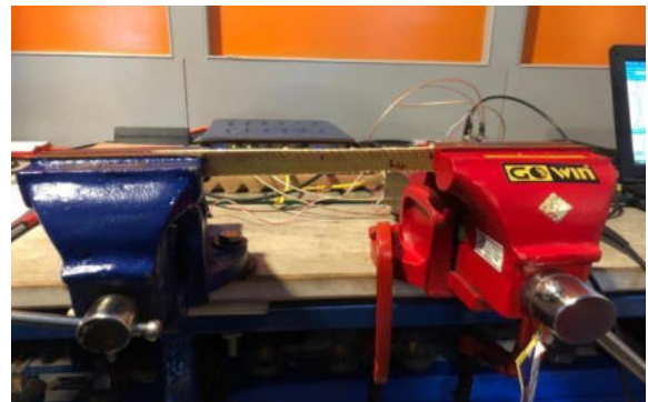
FIG 3.10 LAMINATE 4 OF FIXED-FIXED BEAM
