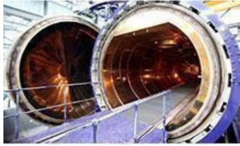
Fig.1.11 An Autoclave at the National Composite Centre.
