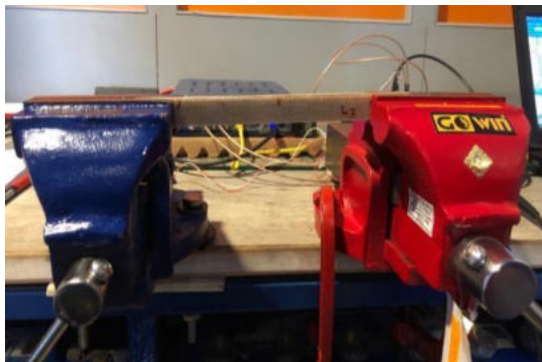
FIG 3.9 LAMINATE 3 OF FIXED-FIXED BEAM
