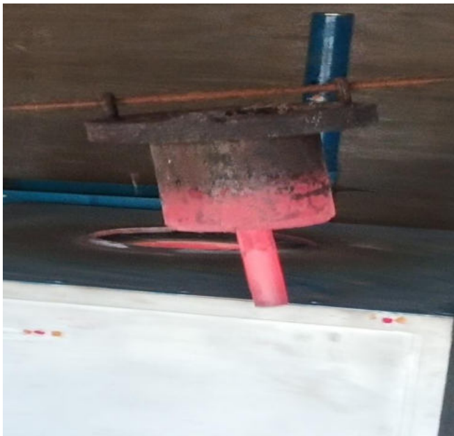
Fig:8 Shows pouring of molten composite into die
