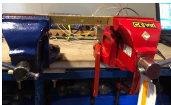
FIG 3.11 LAMINATE 5 OF FIXED-FIXED BEAM
