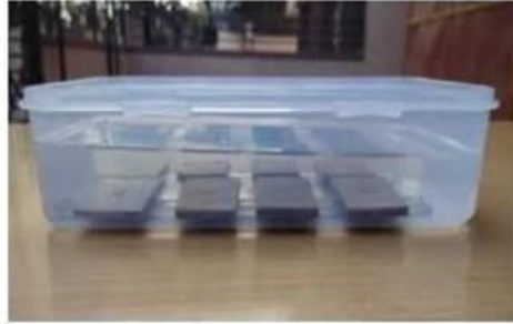
Figure 4.3 – Water absorption test setup
