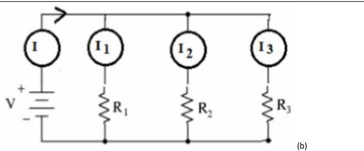
Level 2: Verify KCL with the help of given circuit having # values and carry out the equivalent resistance of the circuit by experimental and analytical methods.
